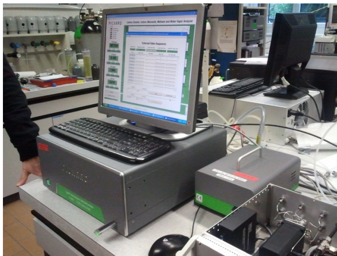
Figure 1.1. Picarro G2401 WS-CRDS instrument at the World Calibration Center for ozone, methane and carbon monoxide of the Global Atmosphere Watch, hosted at EMPA (Zurich)
